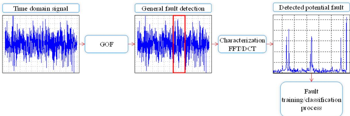
**Figure 1 Classical versus Proposed Fault Diagnosis**
